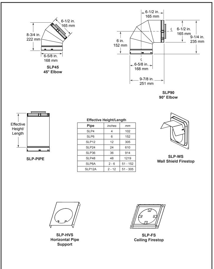
Figure 14.3 SLP Series Vent Components
